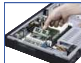
Expendable two Socket-PCI for add-on LAN module
